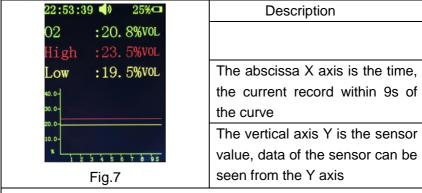
Note: the axis and the data is green, the data curve is blue, the low alarm line is yellow, high alarm line is red.
